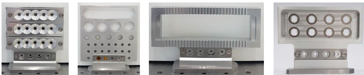
Standard sample holders for: powders, solids, capillaries, and gel/powder samples (left to right)
